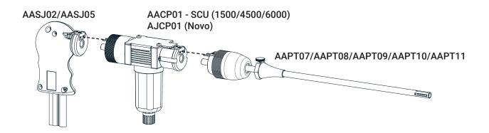
Turn the black probe tip counter-clockwise to loosen and remove the prove tip Simply Plug in the SCU (sample conditioning unit) while matching up the thermocouple and sampling tube. Turn & tighten the metal caps on the SCU and on the removable probe tip to screw the parts together for an air tight connection
