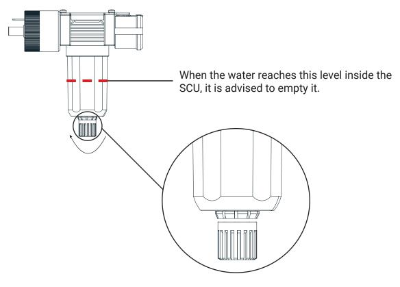
Turn counter-clockwise to remove any condensation after **each** test. Turn clockwise to tighten and close after moisture is drained.
