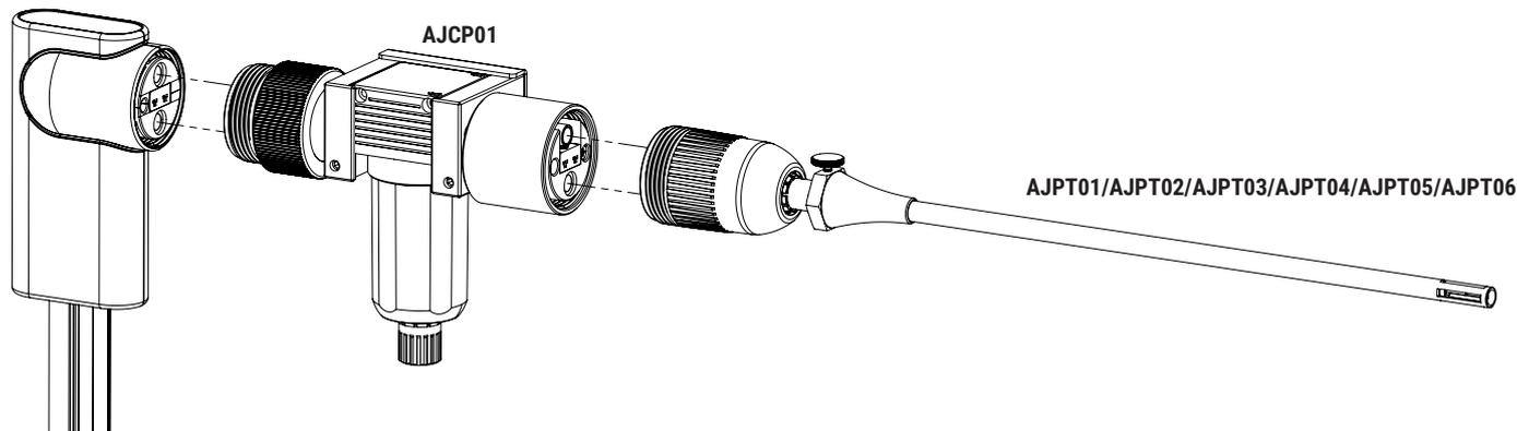
Plug in the handle with the sample conditioning unit matching the thermocouple and the sampling tube. Turn the metal caps on the conditioning unit and on the removable probe tip, so to screw the parts together.
