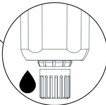
*Turn clockwise to remove any condensation after each test.*
