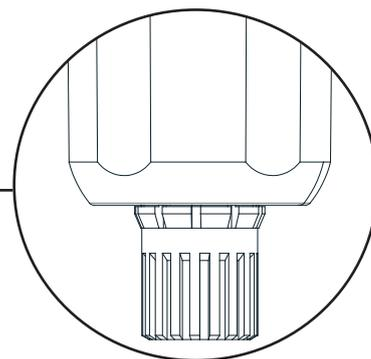
*Turn counterclockwise to close back the cap before starting a new analysis.*
