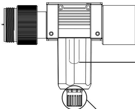
*It is recommended to empty the the water trap when the level of the internal filter inside it is reached by the water.*
