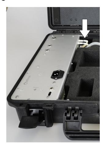
**3** Pull out the rotor of the peristaltic pump, holding inward the two plastic fins indicated by the arrows and at the same time, extract the rotor.
