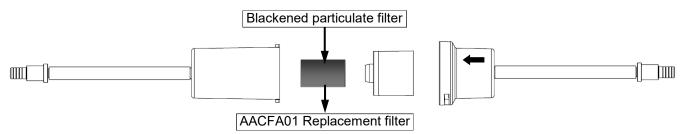
To remove the water trap, just rotate the cover and unhook the filter holder body; remove the internal cup and then replace the filter (see figure).
