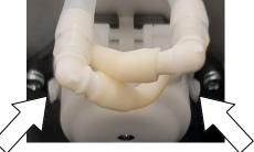
A Remove both tubes from the elbow fittings.
