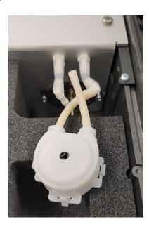
Pulled out the old rotor, replace it with a new one doing reverse operations up to here described, paying attention to the correct insertion of the tubes that must be crossed.
