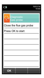
B Start with the sampling probe leak test, which in this case is considered as the tightness test for the whole Cooler system.
