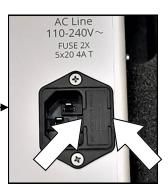
2 Pull out the fuses, with the help of a screwdriver, taking care not to damage the fuse holder drawer and/or the fuses.
