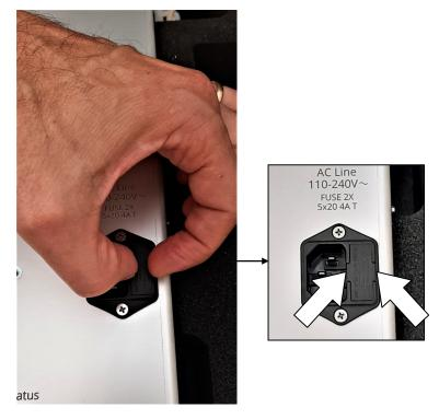
2.Pull out the fuses, with the help of a screwdriver, taking care not to damage the fuse holder drawer and/or the fuses.
