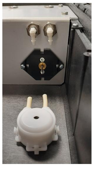
5. Pulled out the old rotor, replace it with a new one doing reverse operations up to here described, paying attention to the correct insertion of the tubes.
