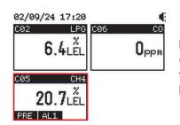
Press the (esc) button to exit the log screen and return to the main screen (which shows the transmitter status panels with concentration measurements). The transmitter that generated the Alarm 1 event is identified with the label "AL1" in the bottom left corner.
