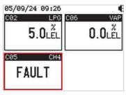
If the conditions that caused the Fault status are no longer present, the controller will turn off the orange FAULT LED and will activate or deactivate the relays and the buzzer depending on how the 'Latch' parameter is configured in the 'Relays' and 'Buzzer' menus for the Fault status. It will also display or not display information on the cessation of the Fault status based on the 'Info event' parameter setting in the 'System => Log' menu.
