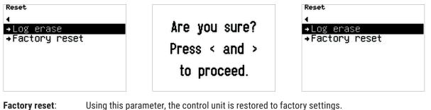
Using this parameter, the control unit is restored to factory settings.
