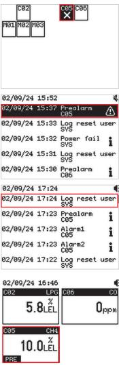
The transmitter that detected an abnormal condition is identified by an "X" on a flashing black background: 🞇, while the others only display the sensor's numerical ID. In the following example, the system has 6 connected transmitters, with transmitter C05 generating the event (in this case, indicating that the pre-alarm threshold has been exceeded).
