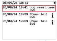
Press the button (esc) 🔊 to exit the log screen and return to the main screen.
