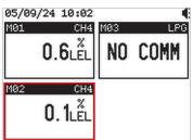
If communication between the transmitter and the controller is restored, the controller will turn off the orange FAULT LED and will activate or deactivate the relays and the buzzer depending on how the 'Latch' parameter is configured in the 'Relays' and 'Buzzer' menus for the Fault status. It will also display or not display information on the cessation of the NO COMM status based on the 'Info event' parameter setting in the 'System => Log' menu.
