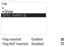
If "Info event" is enabled (flag inserted), when the abnormal event ends, the controller will display information on the log screen about the resolution of the previously detected abnormal event, marked by the icon 1. To exit the log screen and return to the main screen, the operator must reset the events by holding down the button 4 for 3 seconds and then pressing the button (esc) 5. In any case, the events remain recorded in the "Show" parameter for later review.
