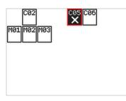
The transmitter that detected the anomaly is identified by an "X" on a flashing black background: , while the others display only the sensor's numerical ID. In the following example, the system has 6 connected transmitters, with C05 generating the event (indicating that the Alarm 1 and/or 2 threshold has been exceeded).
