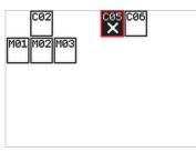
The transmitter that detected the anomaly is identified by an "X" on a flashing black background:  $\mathbf{X}$ , while the others display only the sensor's numerical ID.
