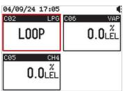
**If communication between the transmitter and the controller is restored,** the controller will turn off the orange FAULT LED and will activate or deactivate the relays and the buzzer depending on how the 'Latch' parameter is configured in the 'Relays' and 'Buzzer' menus for the Fault status. It will also display or not display information on the cessation of the LOOP status based on the 'Info event' parameter setting in the 'System => Log' menu.
