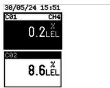
By pressing the arrow buttons, the status panel corresponding to each connected transmitter is selected; first, all transmitters connected to the 4 .. 20 mA inputs (prefix "C") are displayed, followed by all transmitters connected to the RS 485 network (prefix "M").
