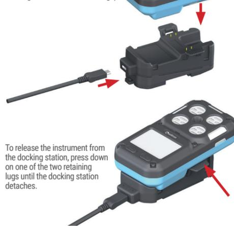
To release the instrument from the docking station, press down on one of the two retaining lugs until the docking station detaches.
