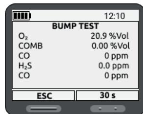
The Bump Test is considered complete within 30 seconds, or when the detector displays the applied gas concentration.
