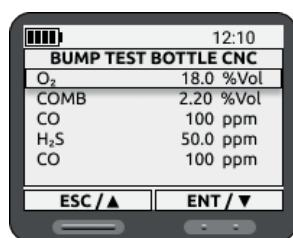
Briefly press one of the two buttons to select the test gas for which you want to change the concentration.
