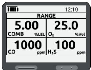
For each measured gas, the screen displays the "LOW ALARM" threshold.
