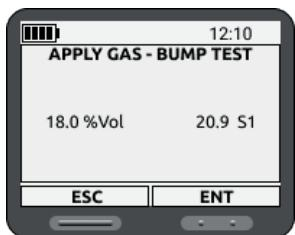
The instrument will display the screen on the side; the test duration is 30 seconds.
