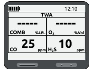
Peak values for each measured gas, recorded since the first use or the last reset, are displayed.
