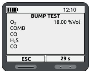
The Bump Test is considered complete within 30 seconds, or when the detector displays the applied gas concentration.
