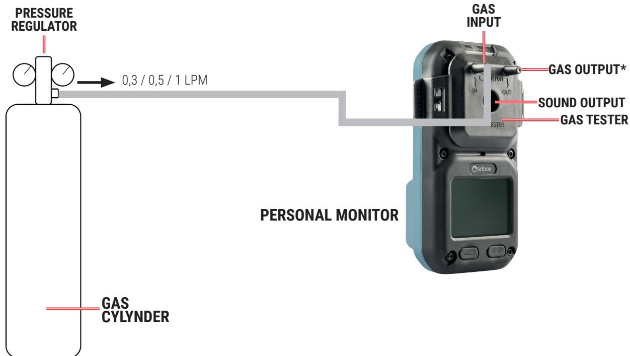
\* From the "Gas Outlet" (OUT) connector, during calibration or BUMP TEST the gas used for the test will come out; for this reason it is absolutely necessary during the use of test gases, to place the instrument inside a fume hood or by means of a tube of the same characteristics as the one supplied, to place the gas outlet remotely.
