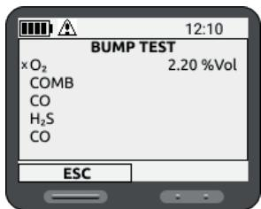
Proceed as described so far to perform the BUMP TEST on the other installed gas sensors.
