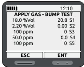
The instrument will display the screen on the side; the test duration is 30 seconds.
