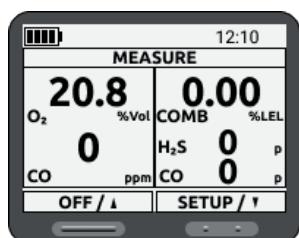
5 display measurements (4 installed sensors including a dual sensor)
