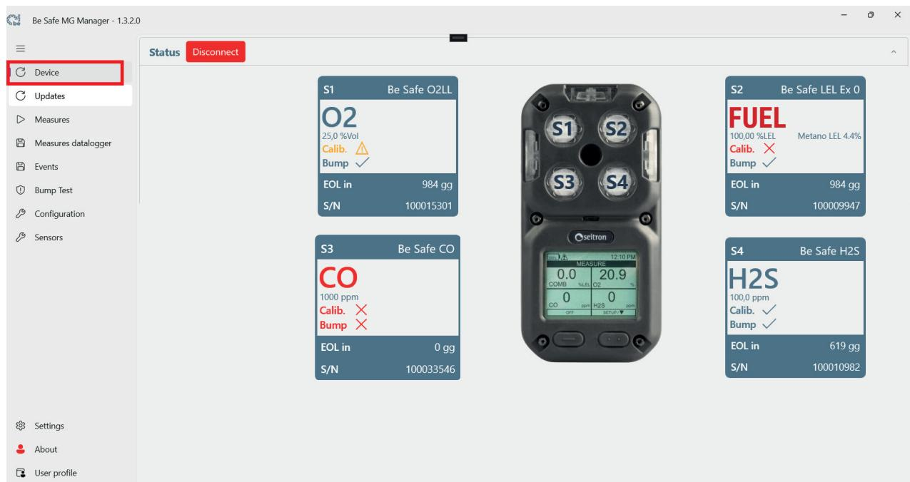
The image of the instrument and the arrangement of the sensors and their status is always visible.
