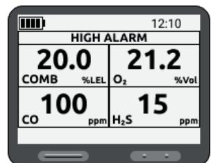
The "STEL" alarms (short-term exposure limit over 15 minutes) for each measured gas are displayed.
