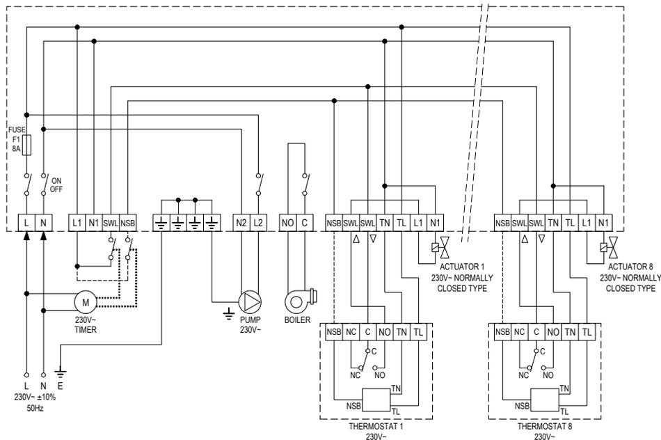
Fig. 4: Wiring diagram.
