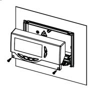
6 ASSEMBLY WITH CABLE INPUT ON THE LOWER SIDE: fit the cable fasteners and/or the blocks delivered with the unit.
