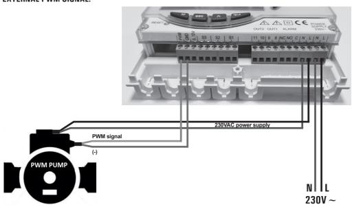
EXAMPLE OF CONNECTION FOR 3-SPEED SOLAR CIRCULATORS WITH WET or "HIGH EFFICIENCY" ROTOR COMPLIANT WITH DIRECTIVE Erp 2015, WHICH DOES NOT REQUIRE AN EXTERNAL PWM SIGNAL (WITHOUT A CONNECTOR FOR PWM).
