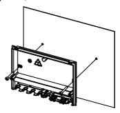
Fit the cover again with the electronics at the base.
