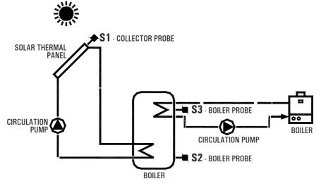
WIRING EXAMPLE ONLY FOR SOLAR CIRCULATORS IN ACCORDANCE WITH DIRECTIVE Erp 2015 WITH EXTERNAL PWM SIGNAL.
