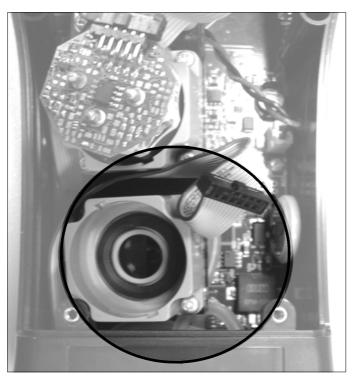
Fit the sensor again taking care the electric connection is turned outside the instrument, not inside (See point 5).
