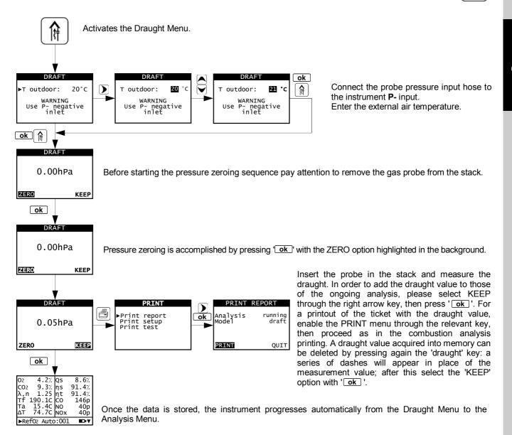
NOTE: The draught values to be stored in the memory must be acquired before performing the flue gas analysis.
