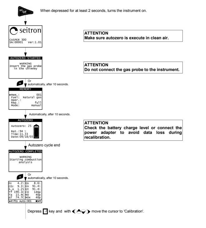
In the following a recalibration example, referred to the CO sensor, is explained.
