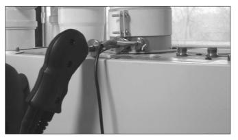
The screw on the cone allows the probe to be stopped at the right measuring depth - this usually corresponds to the centre of the exhaust pipe. For greater positioning accuracy, the user may insert the probe gradually into the pipe until the highest temperature is read. The exhaust pipe must be inspected before carrying out the test, so as to ensure that no constrictions or losses are present in the piping or stack.
