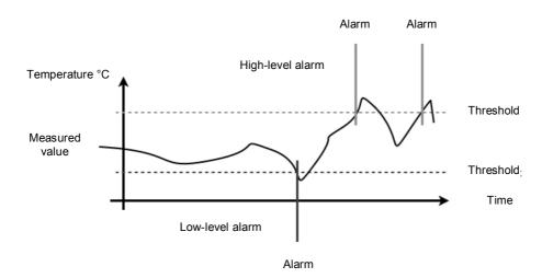
When an alarm threshold is crossed, the instrument emits an intermittent audible alarm besides activating a visible alarm wherein the background of the name of the relative reading will start flashing in the analysis screen.
