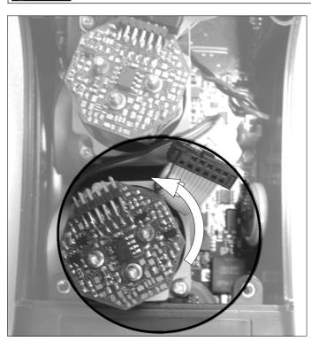
After rotating the sensor, pull it upward; here is an example of the sensor compartment with a sensor removed.
