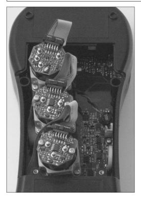
4 Locate the sensor to be replaced; here is an example of a connected sensor to be replaced.
