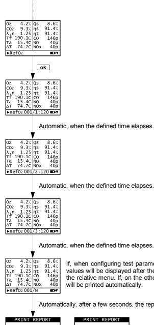
If, when configuring test parameters, manual printing has been selected (see example), the average values will be displayed after the third test values have been read. These may be printed by activating the relative menu. If, on the other hand, automatic printing has been selected, the average test values will be printed automatically.
