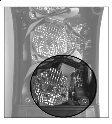
6 The sensor is bayonet-connected to its socket; rotate it anticlockwise to remove it. Here is an example of a rotated sensor.
