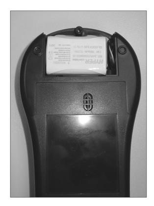
**3** Remove the battery pack connector, and replace the pack with a new one following the reverse procedure described above.
