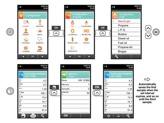
In case the automatic print mode is set then the average analysis printing start automatically. Conversely, after the sampling of the third analysis, the average analysis is shown, so that it can be sent to the printer or downloaded as explained in the following.
