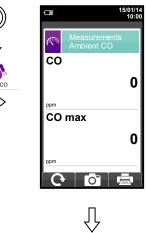
Connect the gas probe to the instrument and perform the measurement. Wait 5 minutes.
