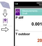
Before zeroing the pressure it is mandatory to extract the probe from the chimney.
