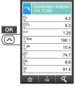
Automatically saves the first sample when the set interval expires, and so on until the third sample.
