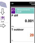
Before zeroing the pressure it is mandatory to extract the probe from the chimney.
