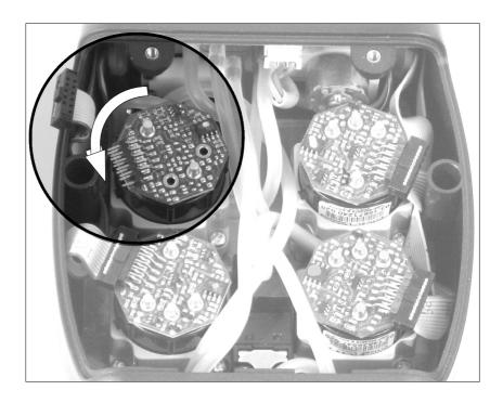
6 After rotating the sensor, pull it upward; here is an example of the sensor compartment with a sensor removed.
