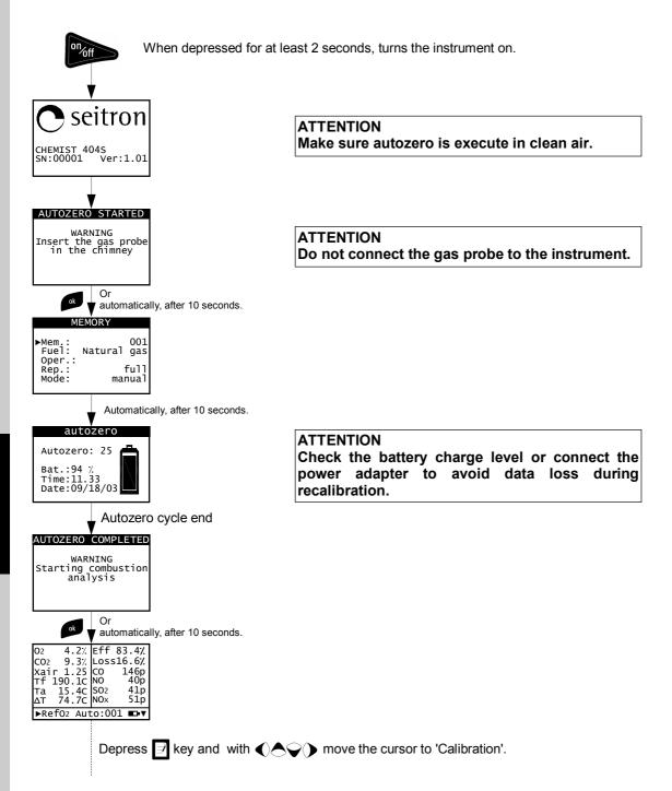
In the following a recalibration example, referred to the CO sensor, is explained.
