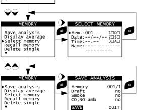
There are 99 storage areas, each of which is capable of storing three test records besides draught, smoke and ambient CO (NO) values. The memory can also be selected from the "Configure Analysis" menu.
