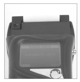
**6** Fit the printer cover taking care to insert the report into the slot on the printer cover.
