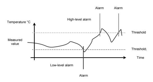
When an alarm threshold is crossed, the instrument emits an intermittent audible alarm besides activating a visible alarm wherein the background of the name of the relative reading will start flashing in the analysis
