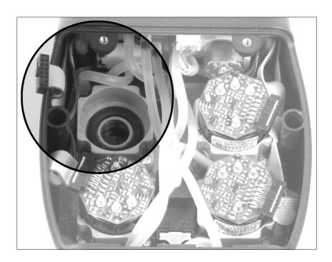
Fit the sensor again taking care the electric connection is turned outside the instrument, not inside (See point 5).
