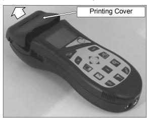
Push inward the plastic thin plate to remove the cover of the paper compartment, as shown by the arrow, until the cover comes out.
