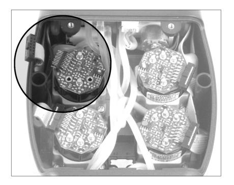
The sensor is bayonet-connected to its socket; rotate it anticlockwise to remove it. Here is an example of a rotated sensor.
