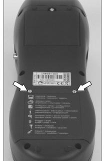
**2** Extract the cover to have access to the sensor compartment.
