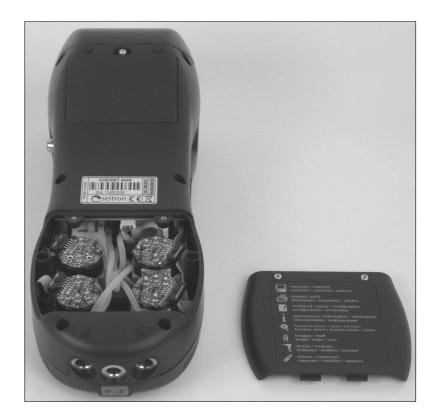
3 Locate the sensor to be replaced; here is an example of a connected sensor to be replaced.
