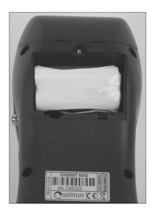
Remove the battery pack connector, and replace the pack with a new one following the reverse procedure described above.
