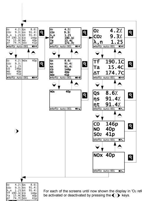
For each of the screens until now shown the display in 'O2 reference mode' (RefO2 is highlighted) can be activated or deactivated by pressing the () keys.
