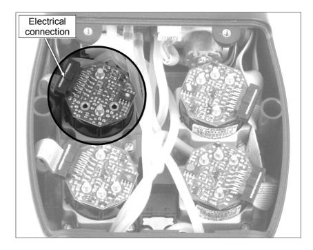
4 Disconnect the sensor to be replaced; here is an example of a disconnected sensor to be replaced.
