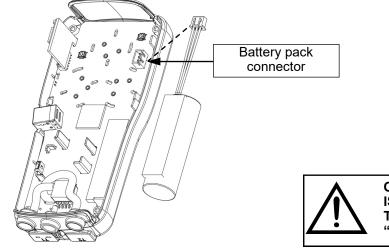
ONCE THE BATTERY IS REPLACED IT IS NECESSARY TO RESET DATE AND TIME THROUGH THE PARAMETER "CLOCK" (<u>SEE CHAPTER 12.3.2</u>).
