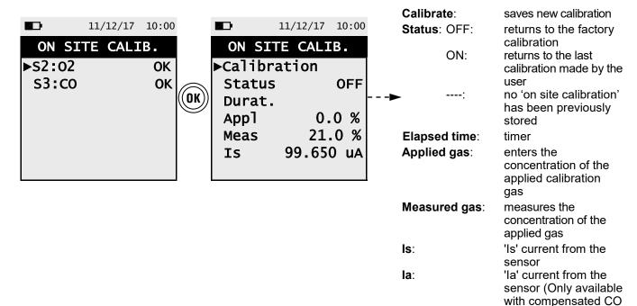
4. In the following a detailed recalibration example will be described for O2 and CO sensors.
