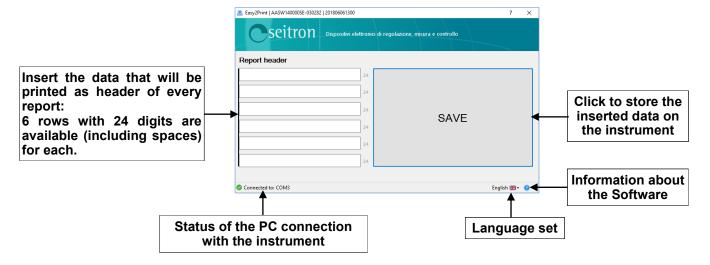
5. By pressing the "SAVE" button, the analyzer will store the inserted data and can be switched off and/or disconnected from the PC.
