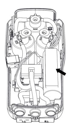
Remove the battery pack connector, and replace the pack with a new one following the reverse procedure described above.
